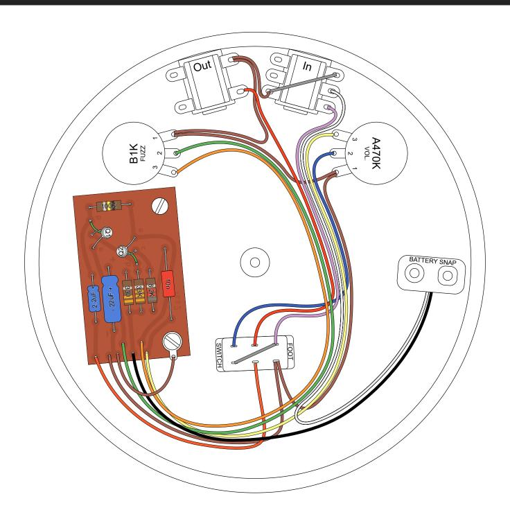
Note: The battery wiring has been updated to use a TRS jack but otherwise all wiring matches vintage units. Check the pinout of your chosen transistors before soldering. Premium style parts kits are are available at <a href="https://www.amplifiedparts.com">www.amplifiedparts.com</a>.
